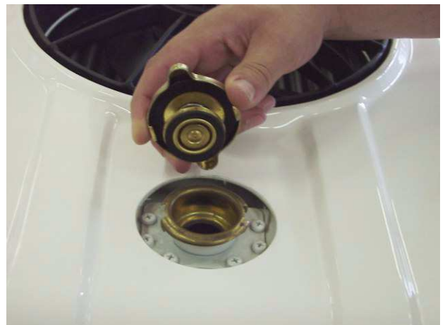
Fig. C.4-5: Cooling water filler neck
