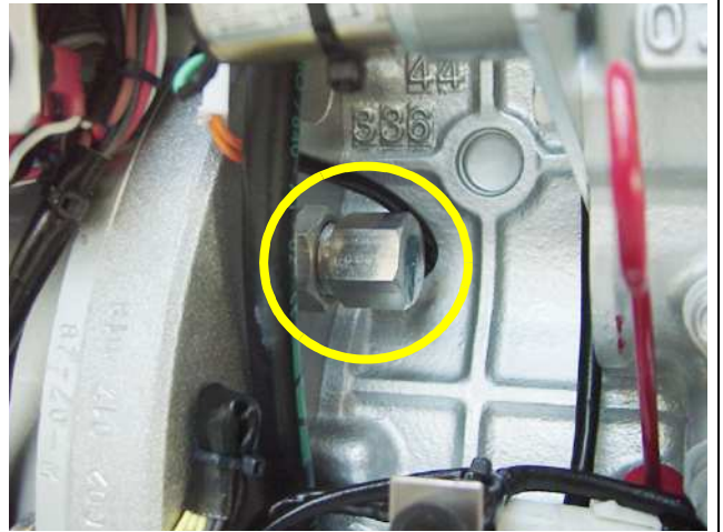
Fig. A.3.5-5: Speed sensor
