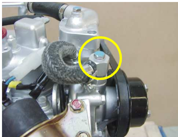
Fig. A.3.2-4: Ventilation screw cooling water pump
