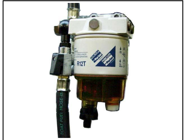
Fig. 9.9-1: Fuel filter with water separator
