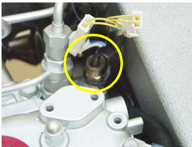
Fig. A.3.6-1: Thermostat at cylinder head
