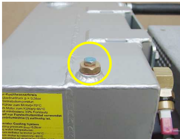
Fig. A.3.2-9: Ventilation screw silencer
