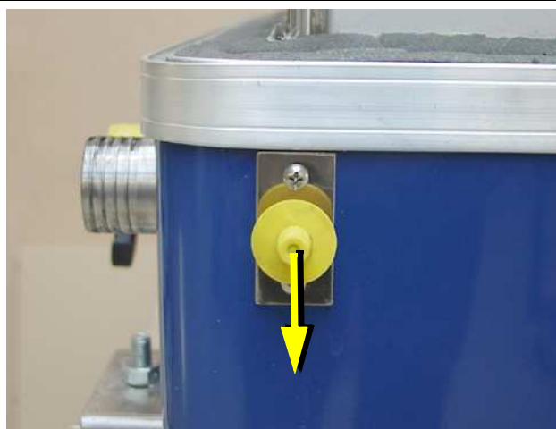
Fig. A.3.2-11: Connection external expansion tank
