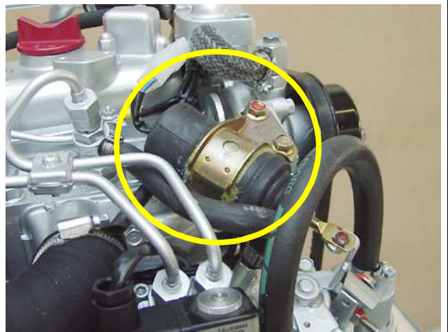
Fig. A.3.3-7: Stop solenoid
