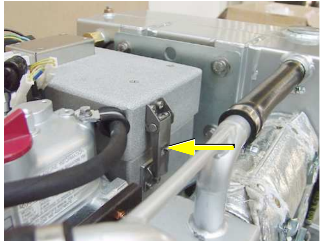
Fig. C.5-2: Airfilter
