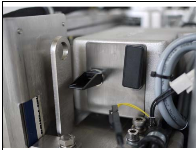
Fig. 9.12.2-2: Air suction housing with pull out holder
