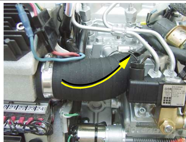
Fig. A.3.4-4: Combustion chamber intake elbow
