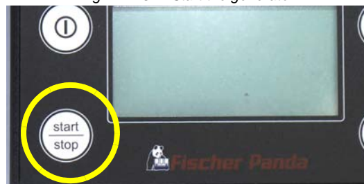
Fig. 14.4.3-2: Start the generator.
