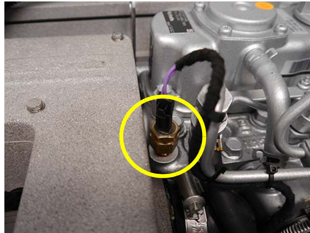
Fig. 6.3.5-1: Thermo-sensor at cylinder head
