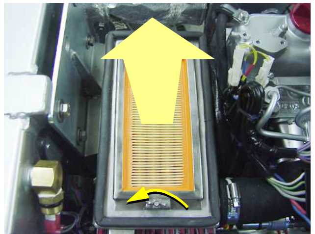
Fig. C.5-3: Air filter mat
