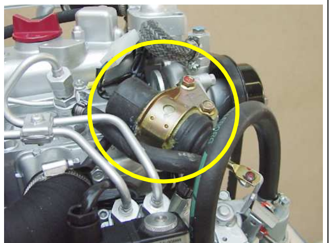
Fig. A.3.5-6: Stop solenoid
