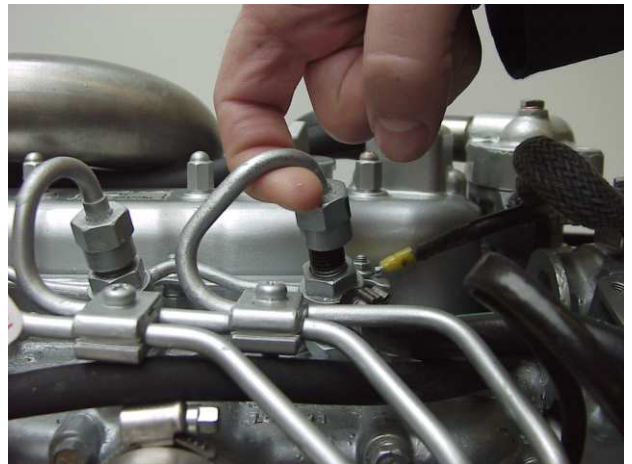
Fig. C.3-4: Injection nozzle
