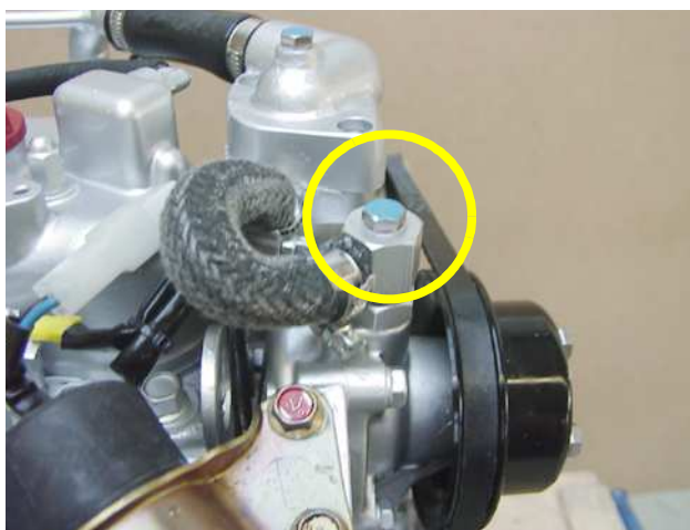
Fig. C.4-1: Ventilation screw
