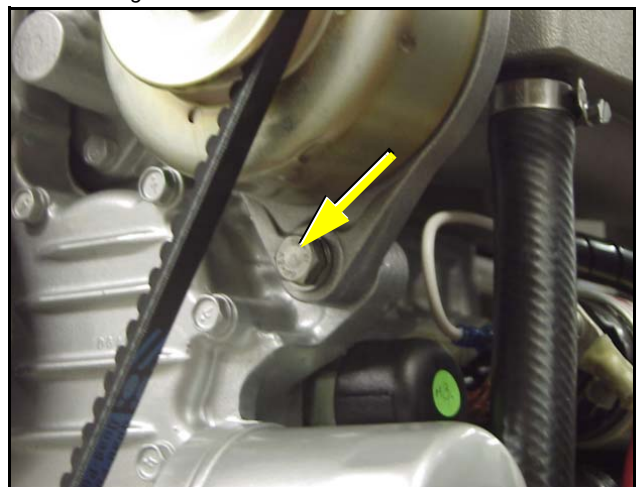
Fig. 9.14-2: Screw underneath the alternator
