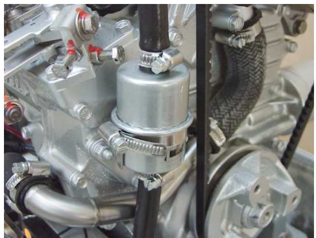
Fig. C.3-1: Fuel filter
