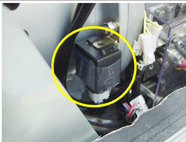
Fig. A.3.5-11: Time relay for stop solenoid
