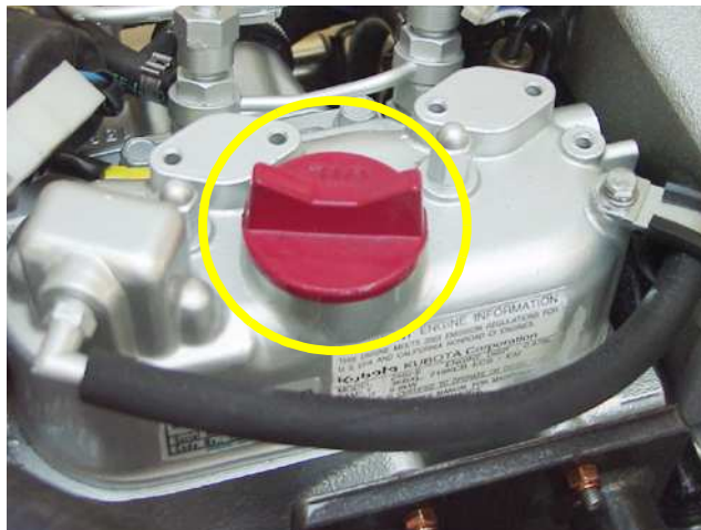
Fig. A.3.7-1: Oil filler neck with cap
