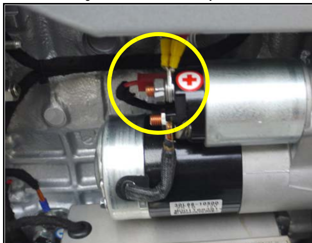
Fig. 8.13.1-1: Positive battery cable
