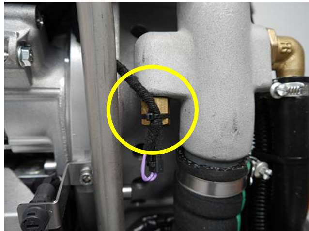
Fig. 6.3.5-2: Thermo-sensor at exhaust connection
