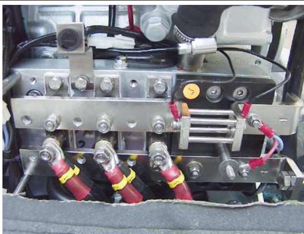
Fig. A.3.5-9: Diode plate
