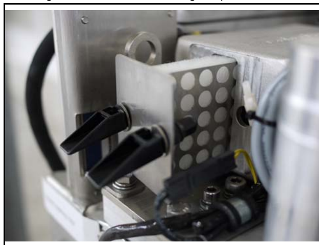
Fig. 9.12.2-3: Air suction housing with pull out holder
