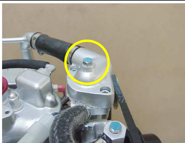
Fig. A.3.2-5: Ventilation screw thermostat housing
