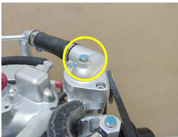
Fig. C.4-2: ventilation screw
