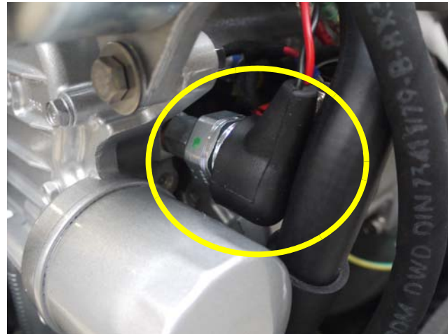
Fig. 3.3.4-4: Oil pressure switch
