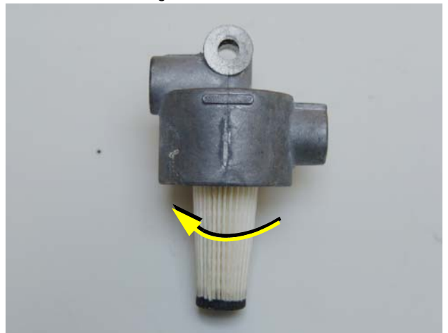
Fig. 6.9.1.1-3: Fuel filter
