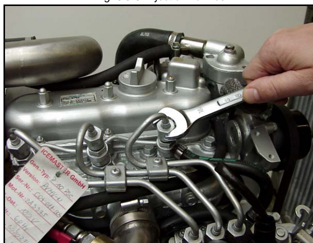
Fig. 6.9-3: Injection nozzles
