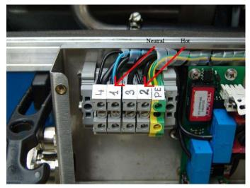
OUTPUT TERMINAL BLOCK LOCATED IN VCS BOX
