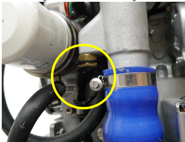
Fig. 4.3.3-5: Thermo-sensor water in
