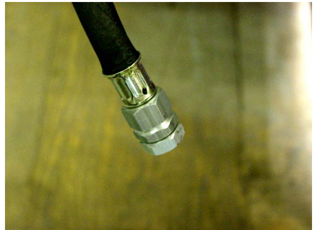
Fig. 7.7-2: Oil drain hose
